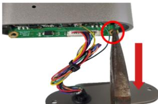
4. Press the hard reset button located on the M/B for 7-8 seconds. The reset takes about a minute to be completed.
