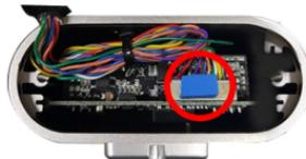
3. Using a plier, grasp the ground hole of the M/B and pull down.
