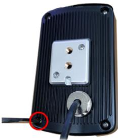
2. Press M/B Factory reset button for 5 seconds
